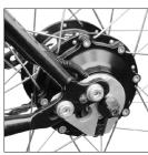
Rohloff SPEEDHUB 500/14 CC OEM mounted in a frame with adjustable Rohloff OEM dropouts
