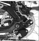
$Rohloff SPEEDHUB \ 500/14 \ A12 \ DB \ PM$  mounted with the  $Rohloff \ PM \ BONE \ (PM-PM \ Adapter)$  and a PM disc brake
