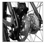
Rohloff SPEEDHUB 500/14 CC DB OEM2 mounted with the Rohloff SPEEDBONE and a disc brake
